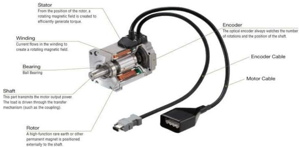
Construction of a standard servo motor
