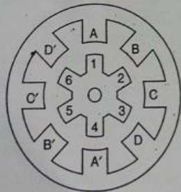
Fig. 1.3 Rotor position when phase A is excited
