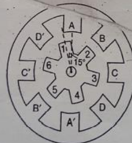
Fig. 1.4 Rotor position when phase B is energised
